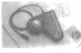
Fig 2-6 The Z mouse features three buttons, a mouse ball underneath, a thumbwheel on the side, and a Trackball on top.
